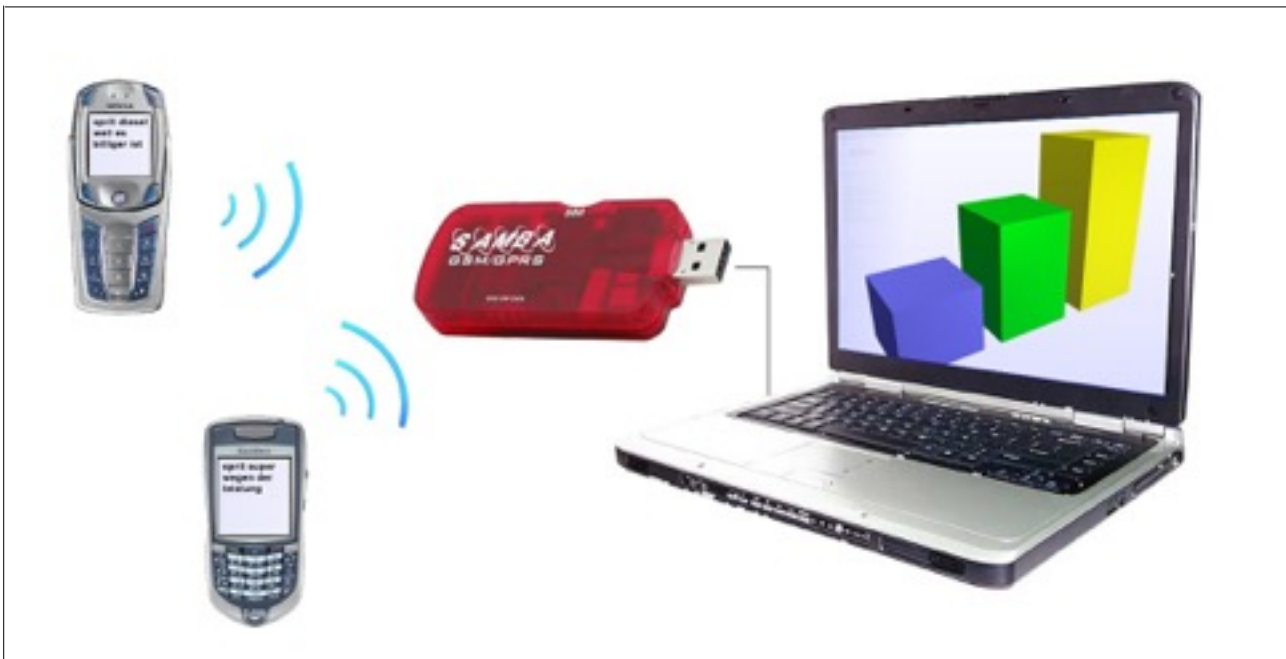
The principle of SMS Voting. The package includes SMS Voting software and a GSM module to receive the SMS.
